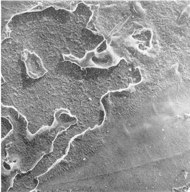
Figure 13 Fracture surface showing biplanar splitting in region F (hesitation line) ( \times 2150 )
