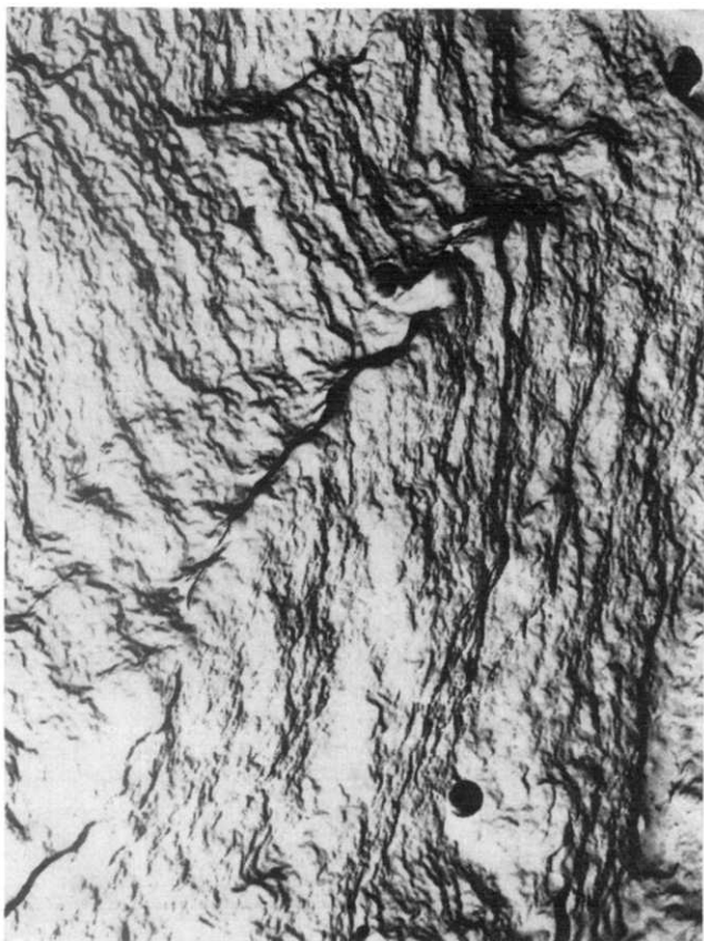
Figure 3. Micrograph of replica of fracture surface of 1,4- trans -polybutadiene. M\eta = 20\ 000 ; T_c = 0^\circ\text{C} .
