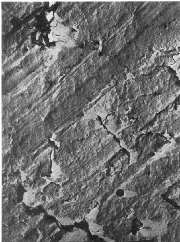
Figure 2. Micrograph of replica of fracture surface of 1,4- trans -polybutadiene. M_{\eta} = 310\ 000 ; T_c = 0^{\circ}\text{C}
