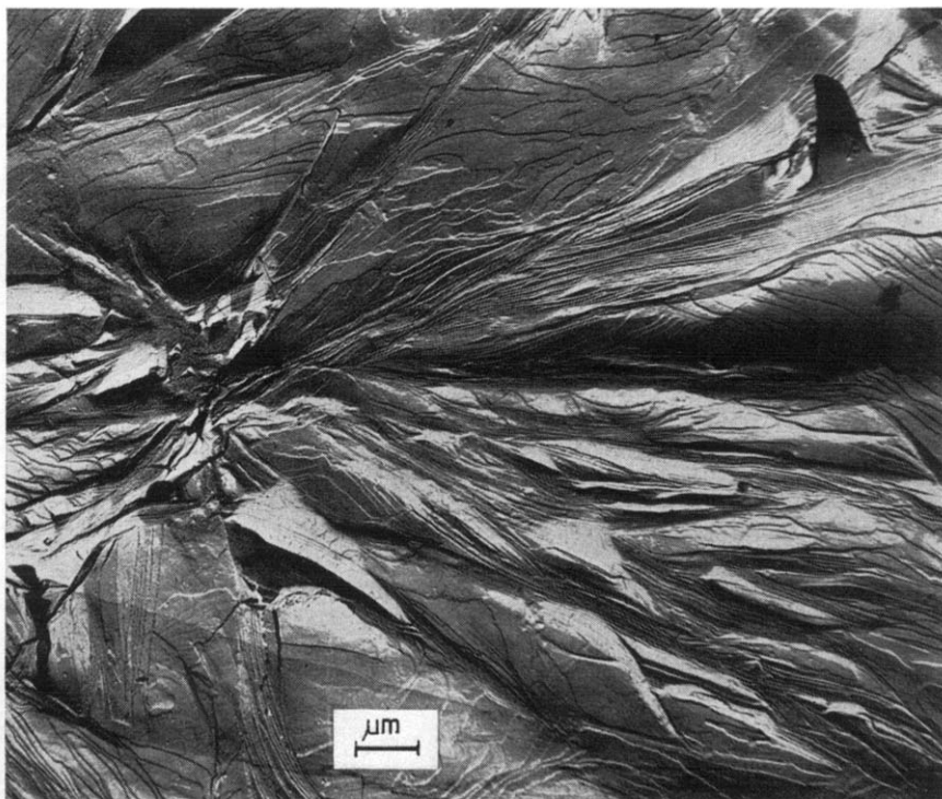
Figure 4 Chain-folded morphology in sample 2 crystallized at 127^{\circ}\text{C} under vacuum for 24 h
